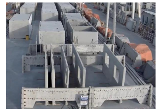
Mobile modular factory -Less labor intensive -Much less cost & fast -Job in time, less messy -higher quality
